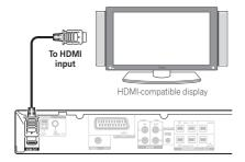
• The arrow on the cable connector body should be face up for correct alignment with the connector on the player.
